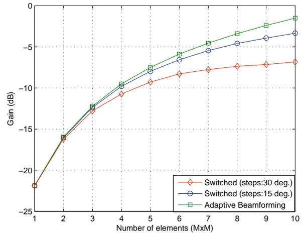
Fig. 2. Gain vs. number of elements in the array (MxM).
