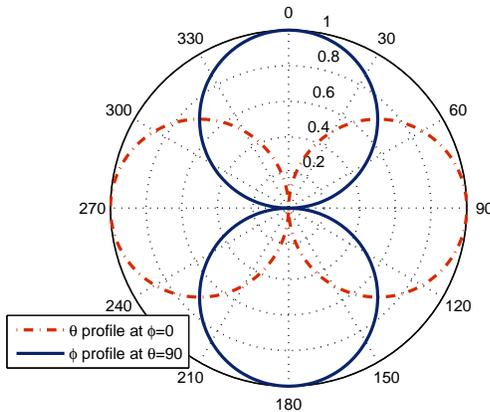
Fig. 1. The radiation pattern each array element.
