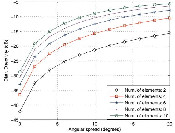
Fig. 6. Distributed directivity vs. angular spread (in both  $\theta$  and  $\phi$  dimensions) of the received signal.
