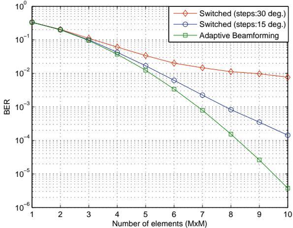
Fig. 3. BER vs. number of array elements ( $M \times M$ ).
