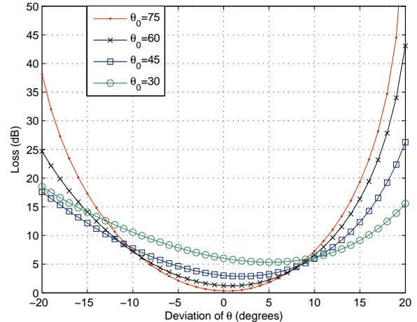
Fig. 4. Loss in power vs. deviation of the received signal from the focus of the beam in  $\theta$  dimension.
