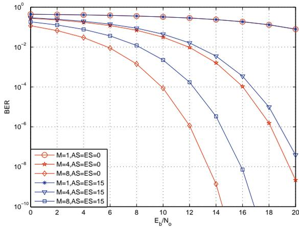
Fig. 7. BER vs.  $E_b/N_0$  for different numbers of array elements with and without angular spreads.
