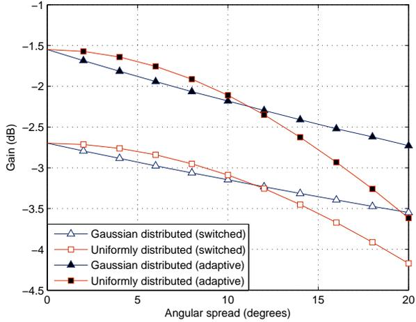
Fig. 5. Gain vs. angular spread (in both  $\theta$  and  $\phi$  dimensions) of the received signal; both Gaussian and uniform distribution cases are plotted.
