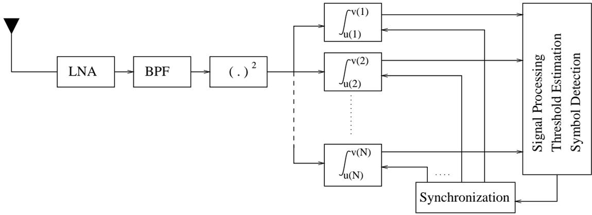
Fig. 1. Adaptive parameter estimation for energy detector receivers.
