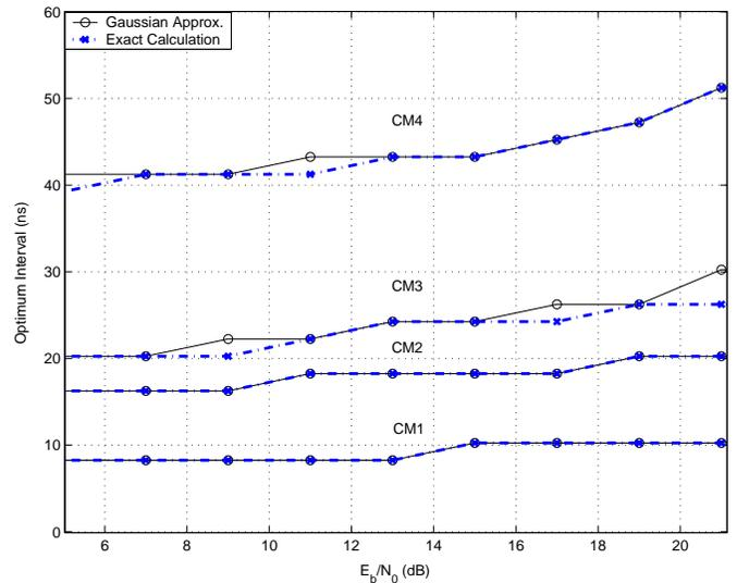
Fig. 5. Optimum integration interval vs.  $E_b/N_0$  for different channel models ( $BW = 2 \text{ GHz}$ ).
