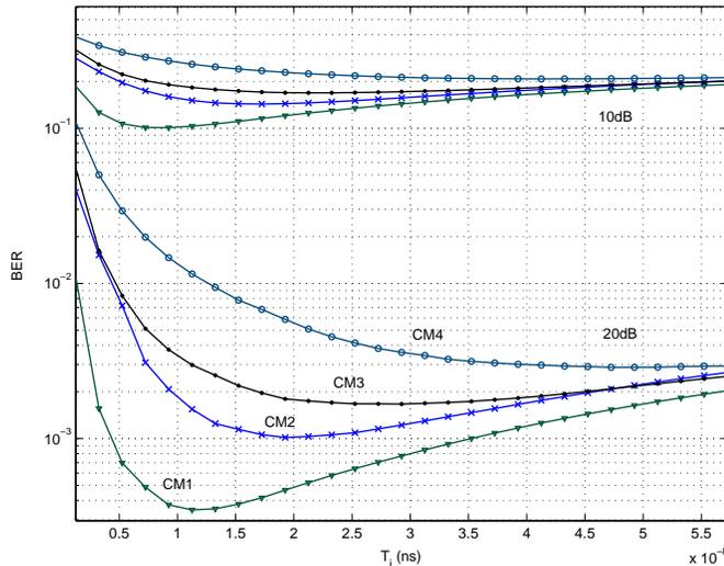
Fig. 4. BER vs. Optimum integration interval for different channel models ( $BW = 2 \text{ GHz}$ ).
