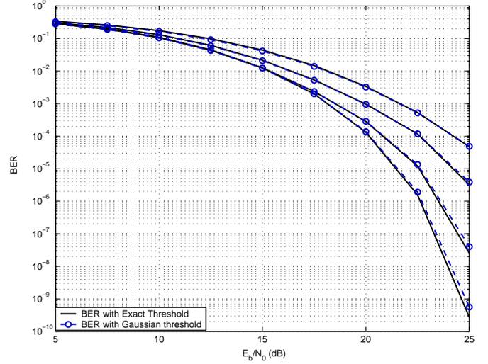
Fig. 2. Bit error rate vs.  $E_b/N_0$  for different integration intervals ( $T_i = 10, 20, 40, 60$  ns and  $BW = 500$  MHz) and for both Gaussian approximated and exact threshold estimates.
