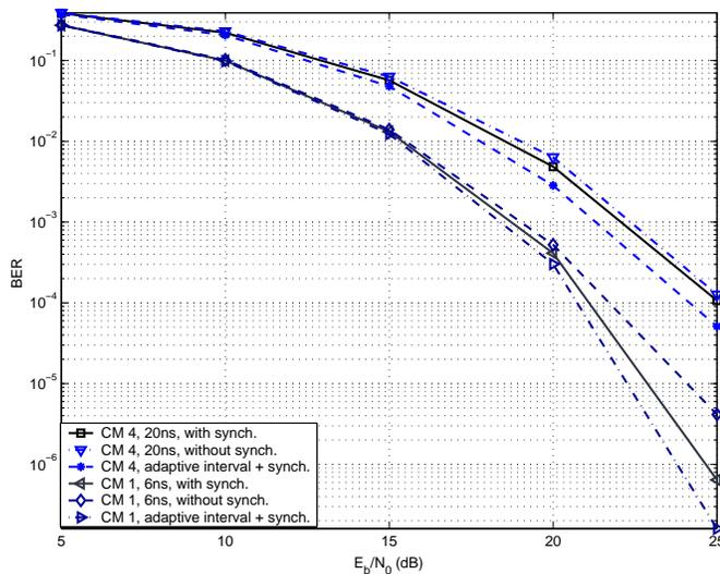
Fig. 3. BER vs.  $E_b/N_0$  for randomly selected fixed integration intervals, adaptive integration interval, and adaptive synchronization point ( $BW = 2 \text{ GHz}$ ).
