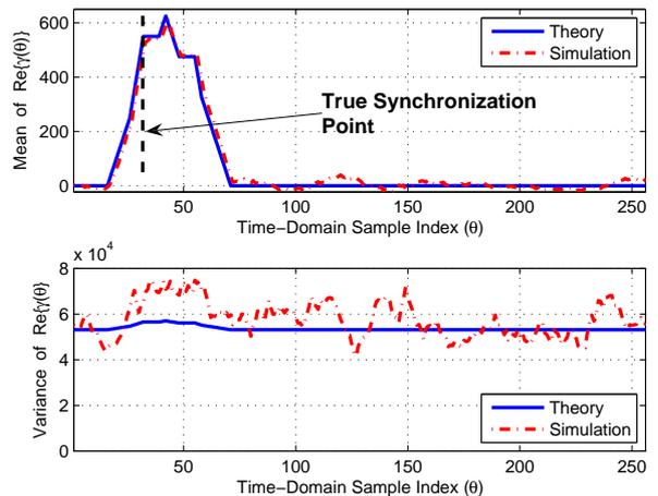
Fig. 5. Comparison of mean and variance of  $\text{Re}\{\gamma(\theta)\}$  for  $D_{\text{max}} = 0$ . Mean of  $\text{Re}\{\gamma(\theta)\}$  is maximized at a sample later than the true synchronization instant.
