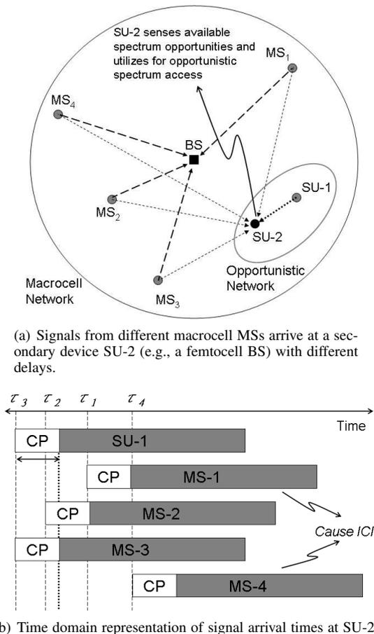
(a) Signals from different macrocell MSs arrive at a secondary device SU-2 (e.g., a femtocell BS) with different delays.
