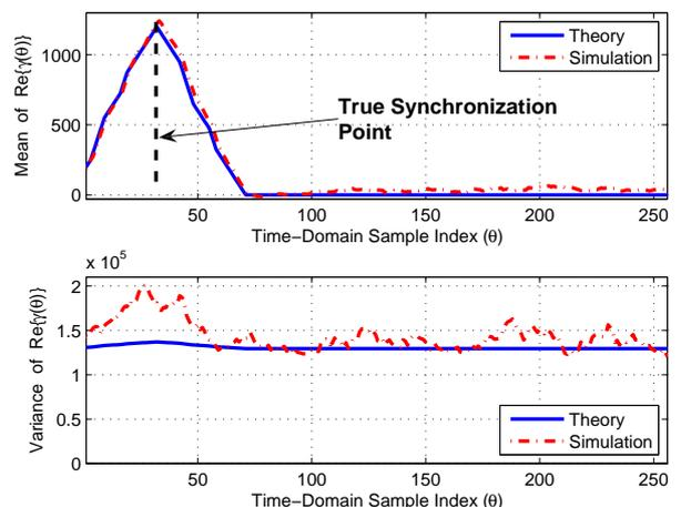
Fig. 6. Comparison of mean and variance of  $\text{Re}\{\gamma(\theta)\}$  for  $D_{\text{max}} = d_3 - d_1 = 23$ . Mean of  $\text{Re}\{\gamma(\theta)\}$  is maximized at the true synchronization instant.
