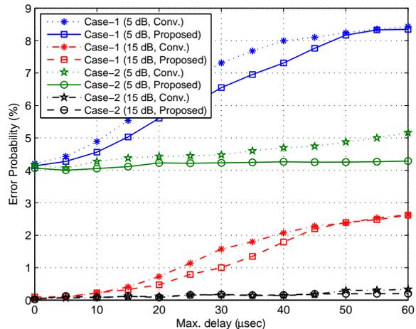
Fig. 7. Performance improvement of spectrum sensing with the proposed synchronization algorithm over correlation based conventional synchronization ( $D_{\max} = 0$ ) and timing misalignment scenarios.
