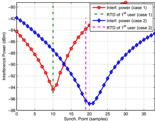
Fig. 2. Effect of the synchronization point on the ICI power. RTD of the first arriving user is close to the optimum synchronization point. Distances of 12 macrocell users to the opportunistic network (in m); case 1: [250, 300, ..., 800]; case 2: [500, 550, ..., 1050].
