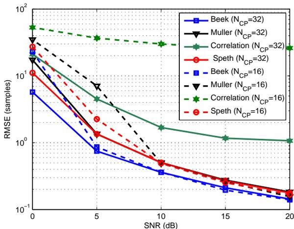
Fig. 3. Comparison of simulated RMSEs of the four different techniques for blind synchronization in a single-user scenario (without averaging).
