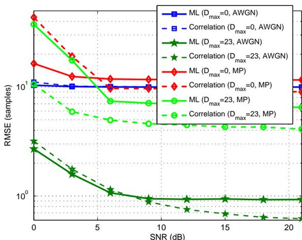
Fig. 4. Comparison of simulated RMSEs of different techniques for blind synchronization in a multi-user scenario ( $N_{\text{avg}} = 21$ ,  $N_{\text{CP}} = 32$ ).
