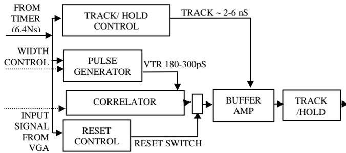
Fig. 5 Correlator Cell Block Diagram
