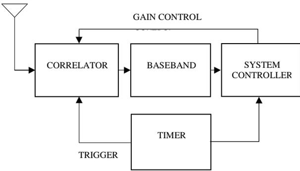
Fig. 3 UWB receiver block diagram
