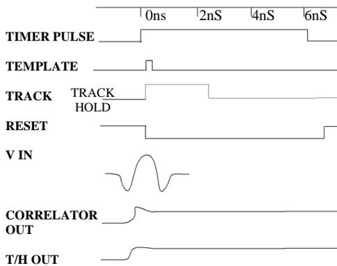
Fig. 6 ASIC Timing Diagram
