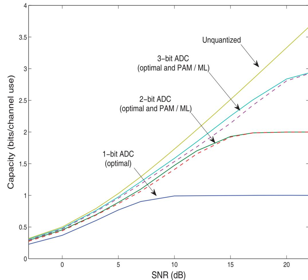
Capacity plots for different ADC precisions in SISO channel (from \*)
